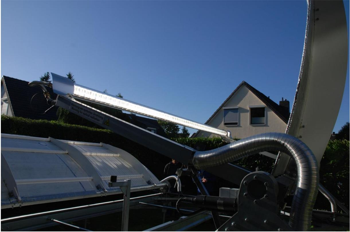
**SunOyster with concentrator cell receiver in operation in Halstenbek near Hamburg, Germany**
